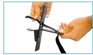
3. Place the T-piece in between the mattress and the boxspring and pull the strap tight so the bed rail is pulled tight against the mattress on the other side. Then feed the strap through the buckle and pull tight again. Lock the buck down and tuck the remaining part of the strap out of the way so it does not become a tripping hazard.
